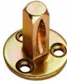
Taylor Spindle (8mm) for fixing handles dead. A Taylor spindle is also known as a Dummy spindle is used where a knob or handle is required to be fixed dead. This means the knob or handle cannot be turned or depressed as per their normal operation. In this manner, the knob or handle are pulled to open the door.
