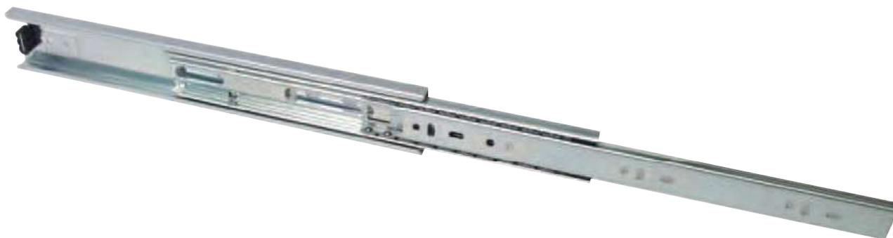
For optimum performance allow between +0.2mm and +0.5mm over the nominal runner thickness, for the runner space.
