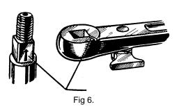
When fitting the arm, ensure that the mark on the arm lines up with the arrow on the pinion, irrespective of the handing of the closer (Fig 6). The exception to this is when the Conversion Bracket is to be installed, when the mark on the arm goes on the opposite side to the arrow on the pinion.
