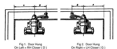
Dimension A, the distance from the centre line of the hinge to the pinion of the closer, varies according to the size of the closer and the required opening angle of the door.
